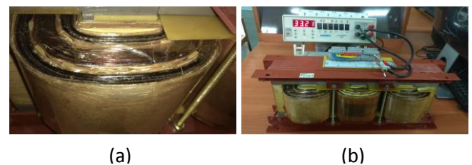
Fig.3 Experimental prototype of 1kW, 415/130 V, 50 Hz delta/zig-zag transformer (a) Top view of winding assembly, showing its rectangular bobbin and spacer arrangement (b) Experimental setup to measure the winding leakage
