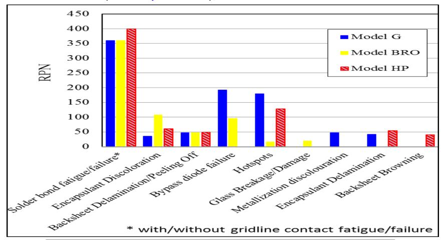
Not all defects are failures:
