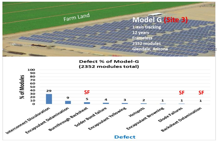
**SF** = Safety Failure; **RF** = Reliability Failure; **DL** = Degradation Loss Defects with safety issues are identified on the plot.
