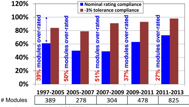
Under-rated modules will show POSITIVE degradation rate Over-rated modules will show OVERLY NEGATIVE degradation rate
