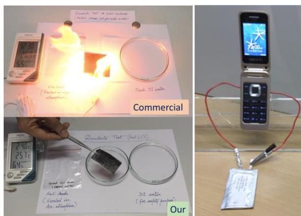
*Fig: The commercial battery that catches fire. Our battery with SnS anode doesn’t catch fire in the same condition.*
